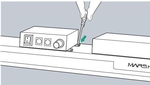
1. Unscrew the four screws on the panel
