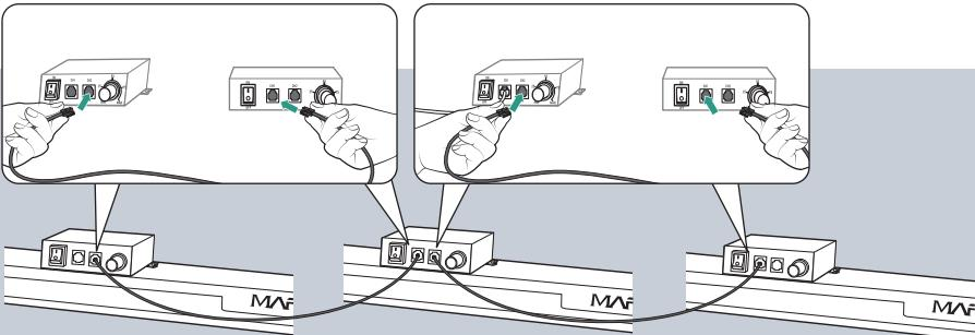
1. Connect multiple lights with dimming cables ( SP3000/SP6500 Support up to 60 lights )
