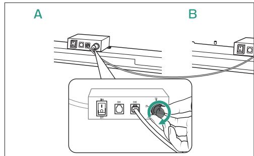
3. Control the intensity of all lights through the dimmer knob of A
